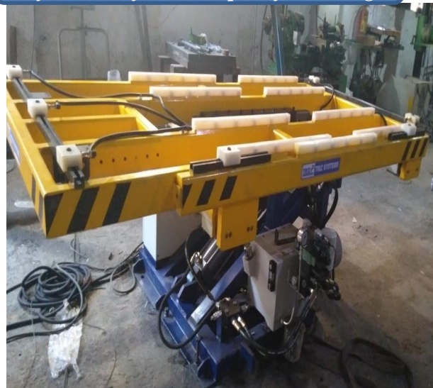
Tilting and rotating Manipulator Hydraulic System– Capacity – 2000kg
