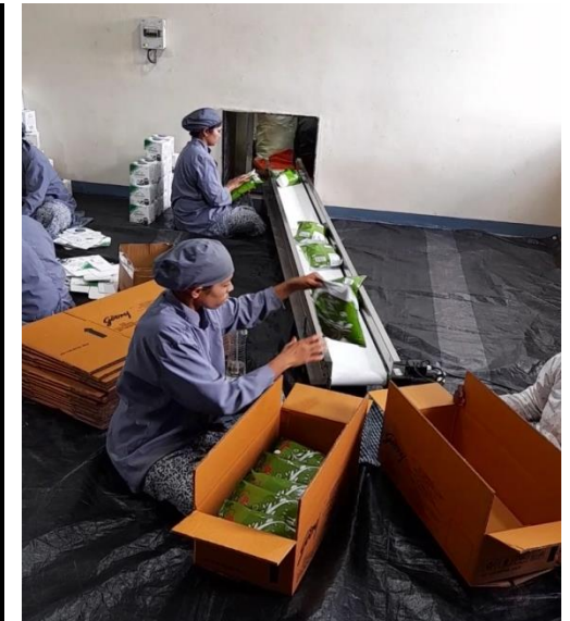
Belt Conveyor For Tea bag Handling
