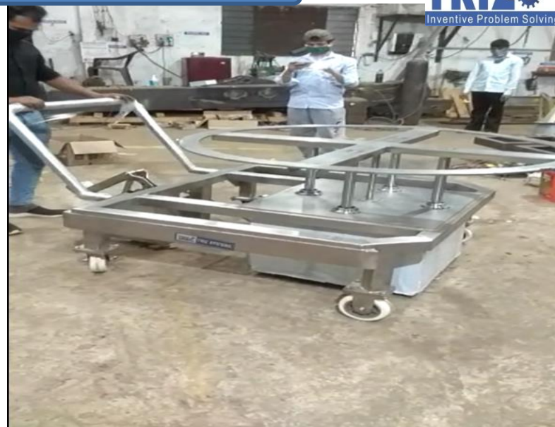
Bottom Disc Lifting Trolley – foot operated , Hydraulic – Capacity -@200 kg
