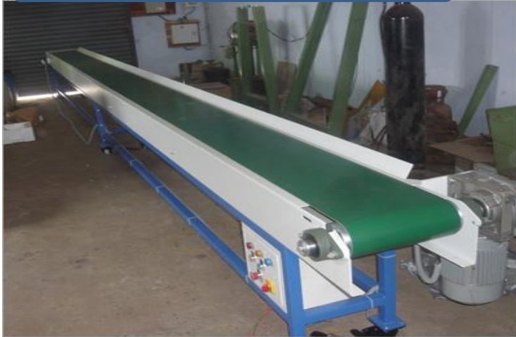
Plane Belt Conveyor – M.S. Structure
