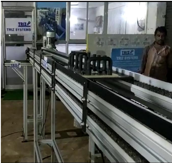
Pallet Handling Chain Conveyors – Power and Free
