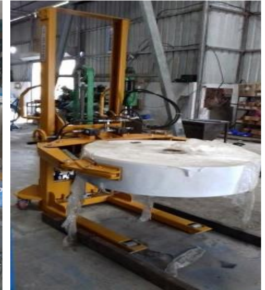
Roll Stackers, Lift and Rotate – upto 1000kg.
