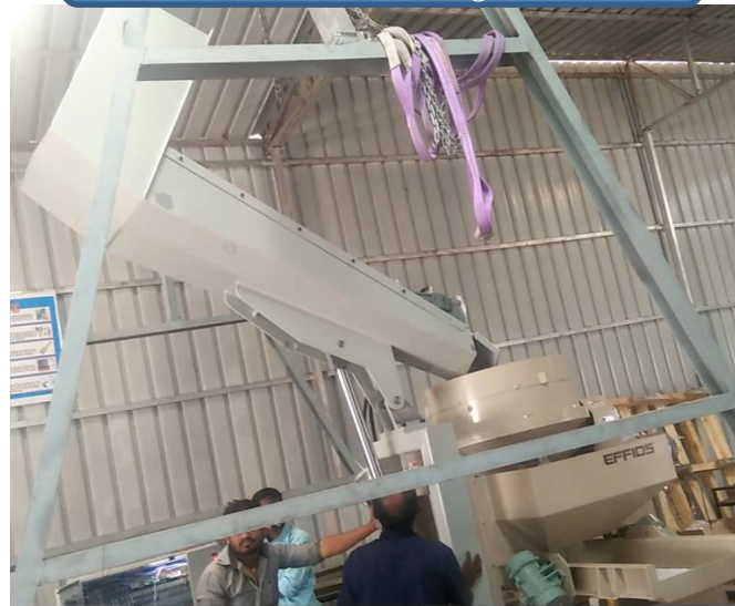
Hydraulic Autoloader by hopper lift and tilt– 500kg
