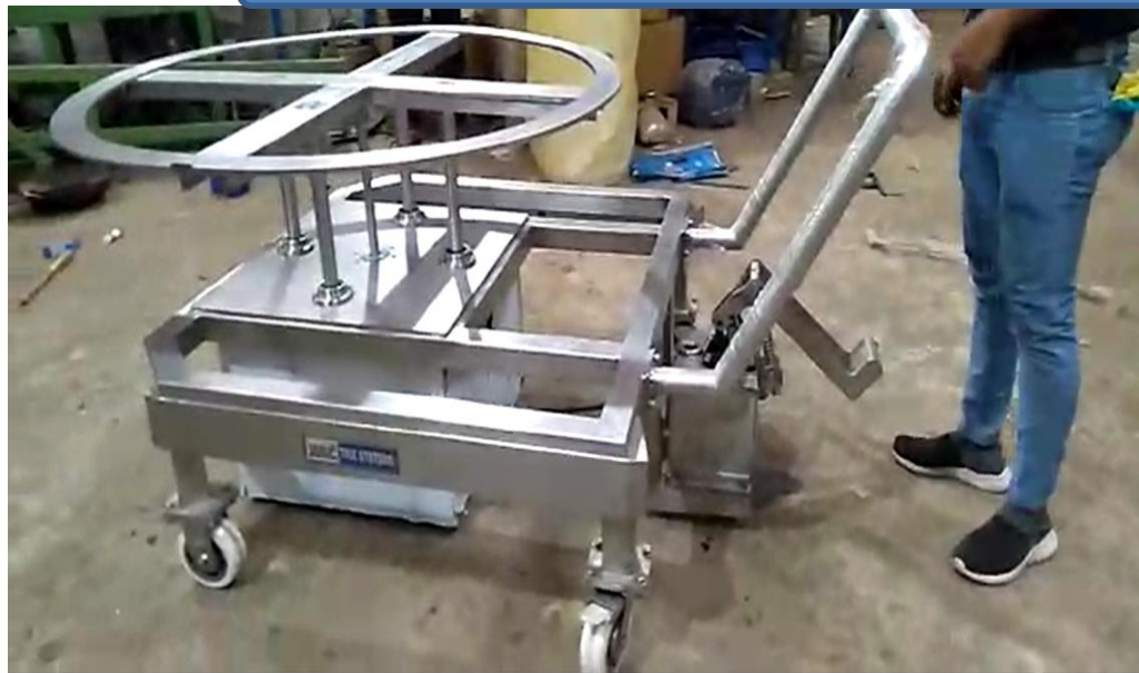
Bottom Disc Lifting Trolley – foot operated , Hydraulic – Capacity -@200 kg
